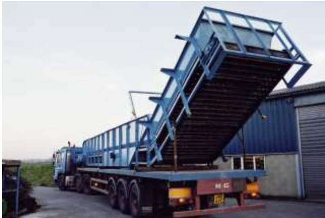
A steel belt conveyor leaving our works destined for installation at Paperchase, Bolton.
