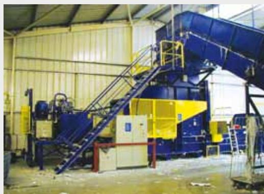
staff to hand-sort the material, 'feed' the baler and then insert the wires to hand-tie the bales. The new equipment can bale the same amount in one hour. It has an automatic tie, which further speeds up the process so the facility consolidates more waste, uses fewer staff, has better tonnages and the compaction ratio is twice as
