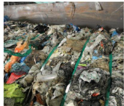
Compacted and baled RDF waste using recycled PET strapping
