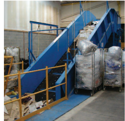
In-floor chain conveyor, with grip top belt and metal flights at Co-operative
