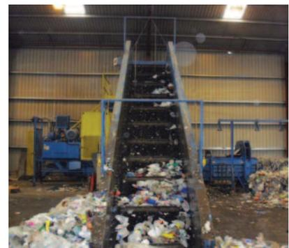
Middleton In floor rubber belt conveyor working
