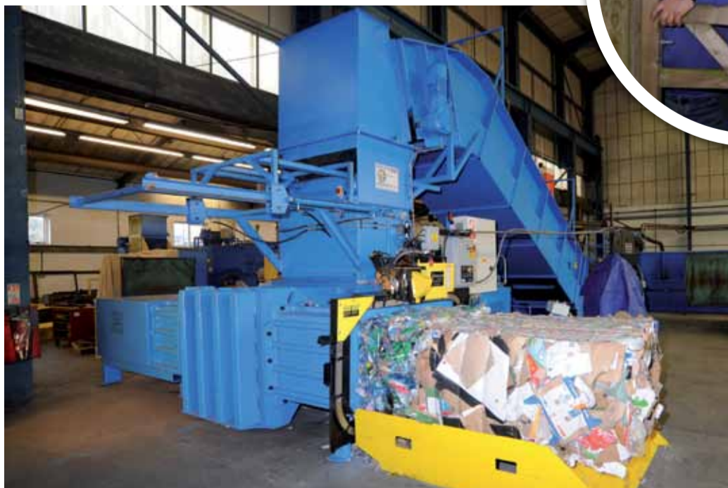
Above: Middleton's twin ram baler being tested. Inset: Ashley and Joan Middleton who founded the company in 1975 and who are both still active at the Gloucestershire-based engineering business
